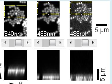
This is caused by chromatic aberration. The reflection is at 488 nm and the multiphoton excitation is at 840 nm.
